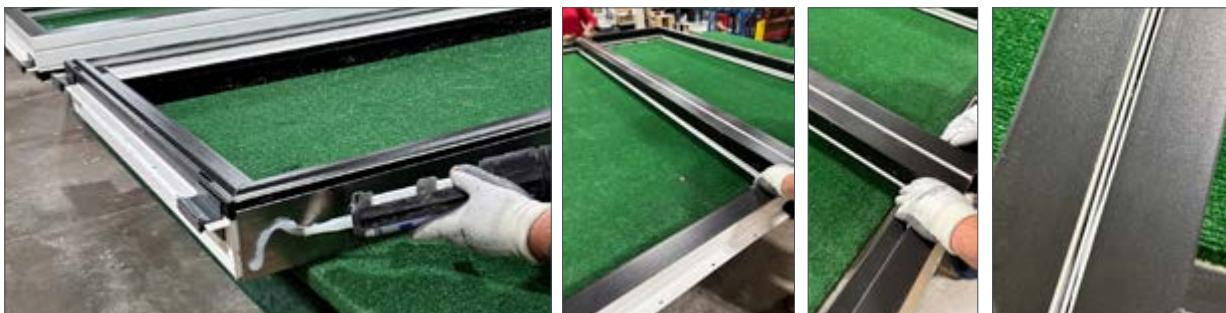
**C.** Clip the corners of the provided mull cover to a 45 degree angle. Then place the mull cover of the mull and gently tap it into place with a rubber mallet from one end to the other.
