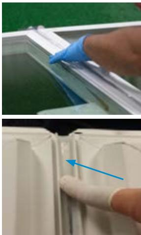
»-Using glove or finger cot, tool silicone smooth across mull bar and into corners.
