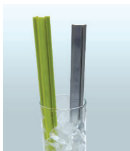
Innergy and Alluminum in a 32 degree ice bath
